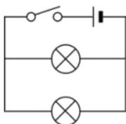
The circuit diagram shows a circuit with two lamps connected in parallel. If one lamp breaks, the other lamp will still light.
