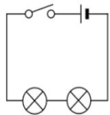
The circuit diagram shows a circuit with two lamps connected in series. If one lamp breaks, the other lamp will not light.
